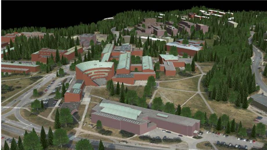
**Figure 2.** Accurate 3D modelling of Helsinki University campus area created from laser scanning data and digital aerial photos.
