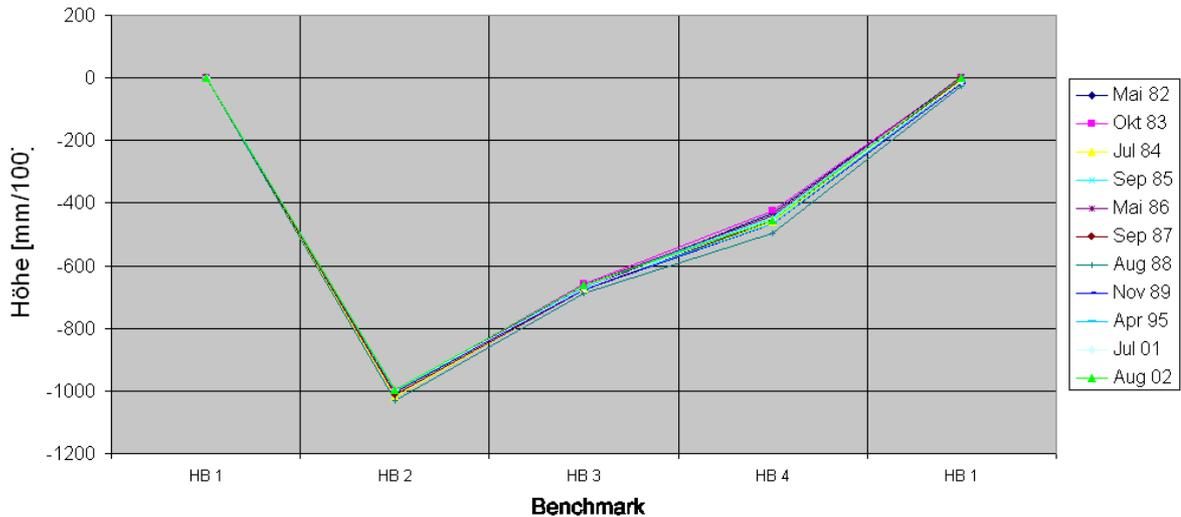
Fig. 4: Results of control levelling around pillar 22 i.e.
