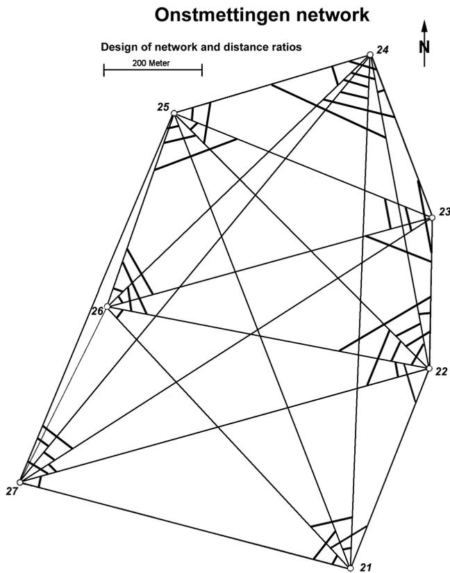
Fig. 3: The design of Onstmettingen network and the configuration of used distance ratios.
