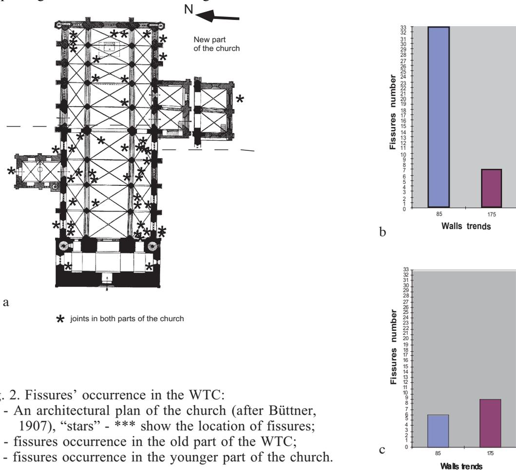
Fig. 2. Fissures' occurrence in the WTC:
