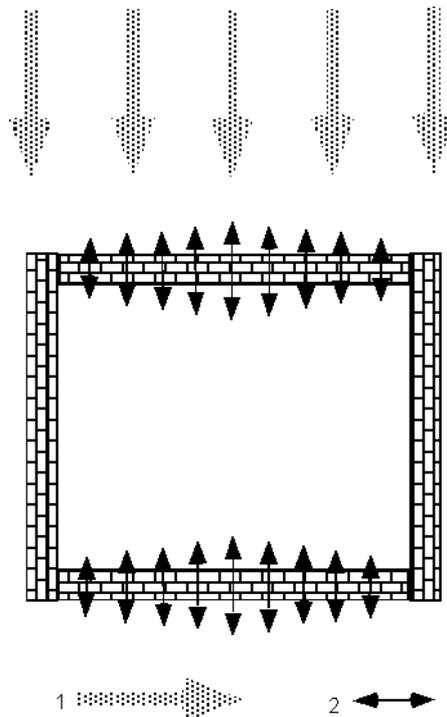
Fig. 5. Different freedom of oscillations (2) for walls with different trends, exposed to seismic movements (1).
