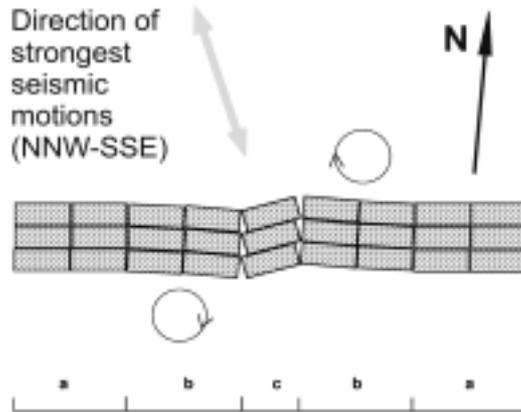
Fig. 3. Rotations in Wittstock church's tower: a model explaining observed rotation pattern. a - undeformed wall, b - parts of the wall underwent clockwise rotations, c - transitional zone of drag (counterclockwise) rotation.
