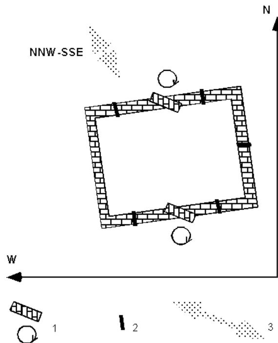
Fig. 6 A model explaining the observed damage patterns in upper part of the Wittstock church. 1 - clockwise rotations, 2 - through-going joints, 3 - axis of the seismic movements
