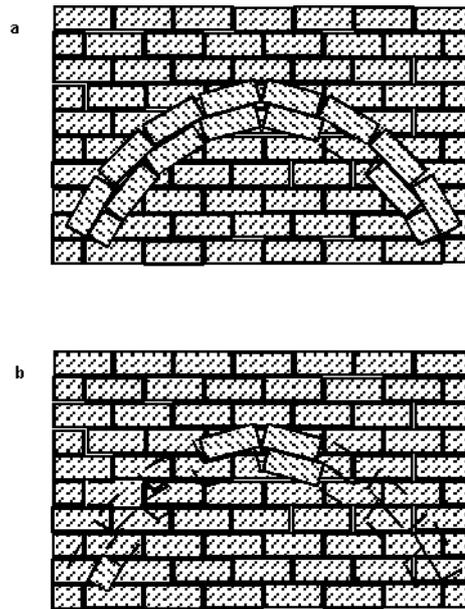
Fig. 4. Different degree of damage of attached arches in the walls with different trends in upper part of the Wittstock church's tower. a - walls trending  $170^{\circ}$ - $175^{\circ}$ , b - walls trending  $80^{\circ}$ - $85^{\circ}$ .
