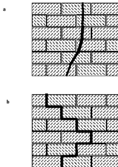
Fig. 1. Different types of fissures in the damaged walls: a - through-going joints, supposing their seismic origin, b - orthogonal cracks, which can be produced by the static loading or seismic oscillations.
