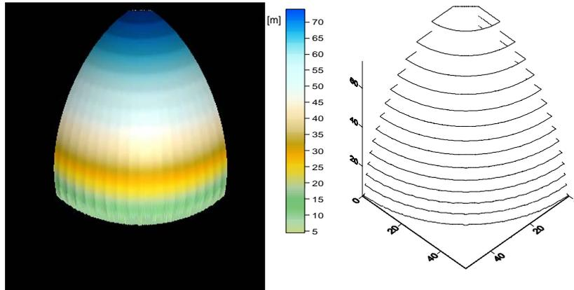
**Fig.2:** Surfaces with the same uncertainty in point position - Surfer 8 software
