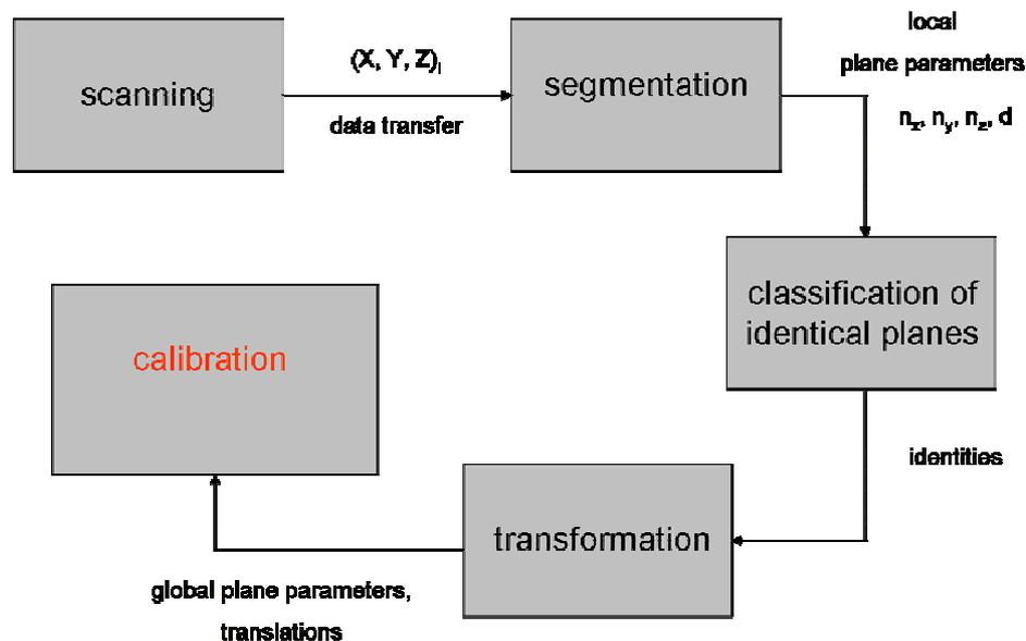
Fig. 4: Overview over the Calibration Procedure
