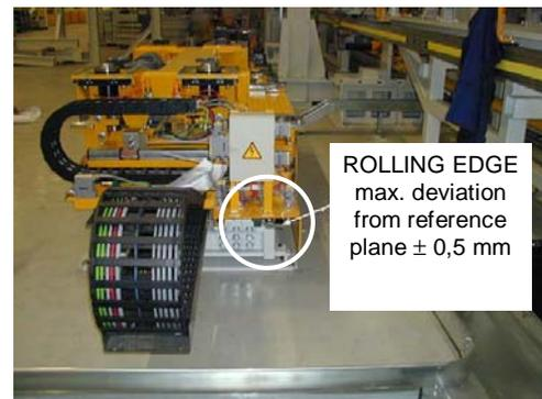
**Fig. 3:** Position of rolling strips
