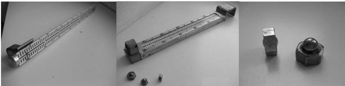
**Fig. 5:** Special measuring staffs and bolsters
