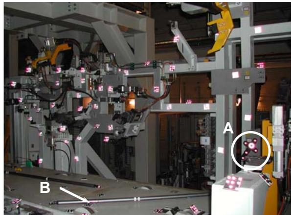
**Fig. 6:** location of markers on the frame.
