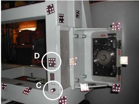
**Fig. 7:** Detail of CYTEC mounting device for fitting of the frame to main table
