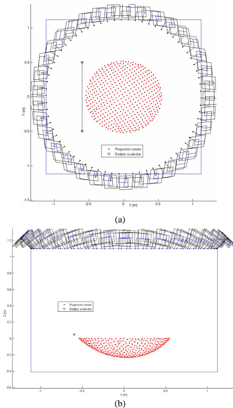
Figure 2. Network configuration. (a) XY-view (aperture of SR) and scale-bar at the left side (b) XZ-view of the network.
