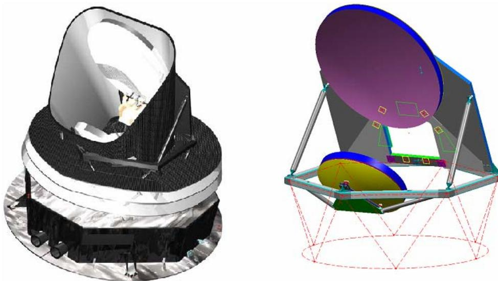
Figure 1. Planck Telescope. Receiving system with the Primary (top) and the Secondary (bottom) Reflectors (Courtesy of Alcatel Alenia Space).
