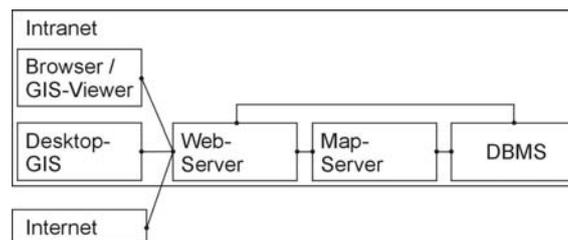
Figure 5. Overall concept for IT system
