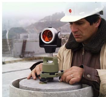
Figure 5 – Tacheometer TCA2003    Figure 6 –Retroreflector GPH1P
