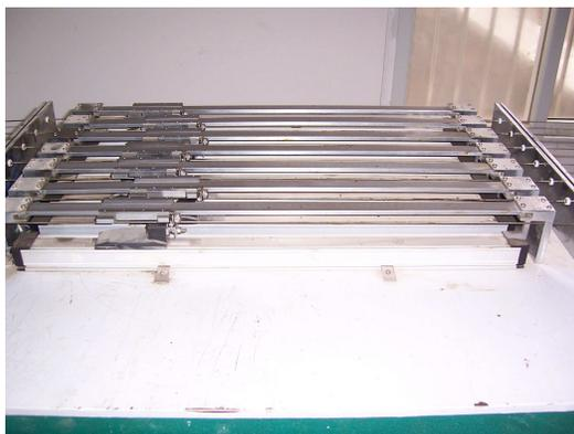
Figure 3 - Interior wire extensometer.
