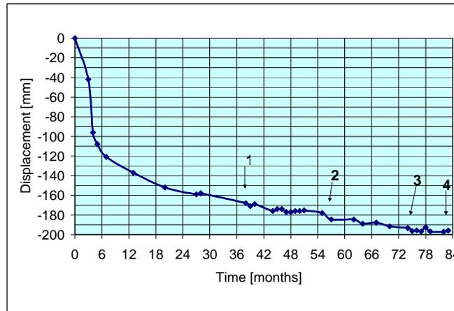
Figure 4 - Measured settlement of point SP4 as a function of time
