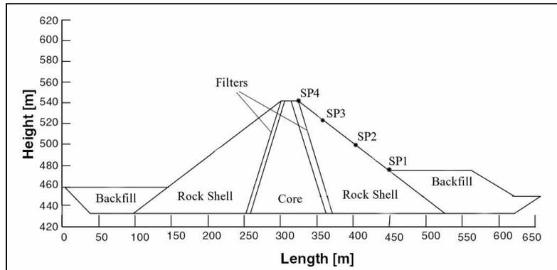
Figure 3 - West Dam cross section
