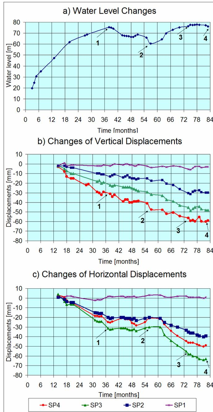
Figure 5 - Water level and displacement changes as a function of time
