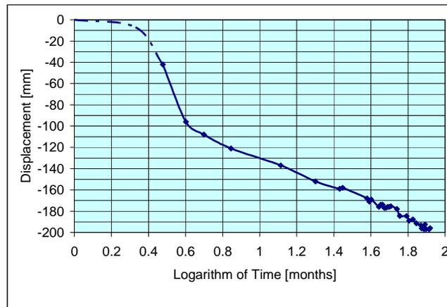
Figure 5 - Measured settlement of point SP4 as a function of log (time)
