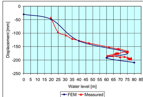
Figure 6 - Modeled and measured settlement of pt. SP4 as a function of water level
