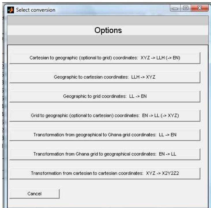
Figure 6 - The graphical display of the options provided in the Ghana Geo-System
