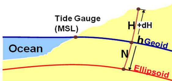
Figure 4 - Diagram showing the relationship Geoid, Ellipsoid and the Geoid Separation
