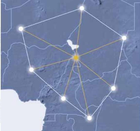
A map of the African continent is shown with a network of CORS (Continuously Operating Reference Station) stations. The stations are represented by white dots, and they are interconnected by a network of lines. A central station is highlighted with a yellow dot, and lines radiate from it to other stations across the continent. The map is overlaid on a blue background with a white grid pattern.
