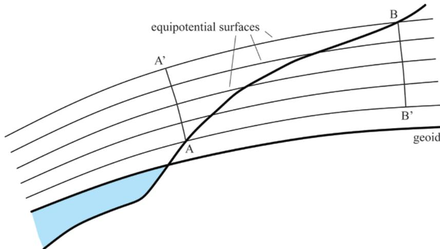
**Figure 1. Non-parallelity of equipotential surfaces**
