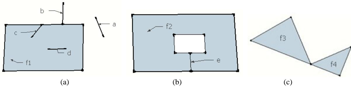
Figure 7. Hanging and dangling edges (a) and redundant edge (b)
