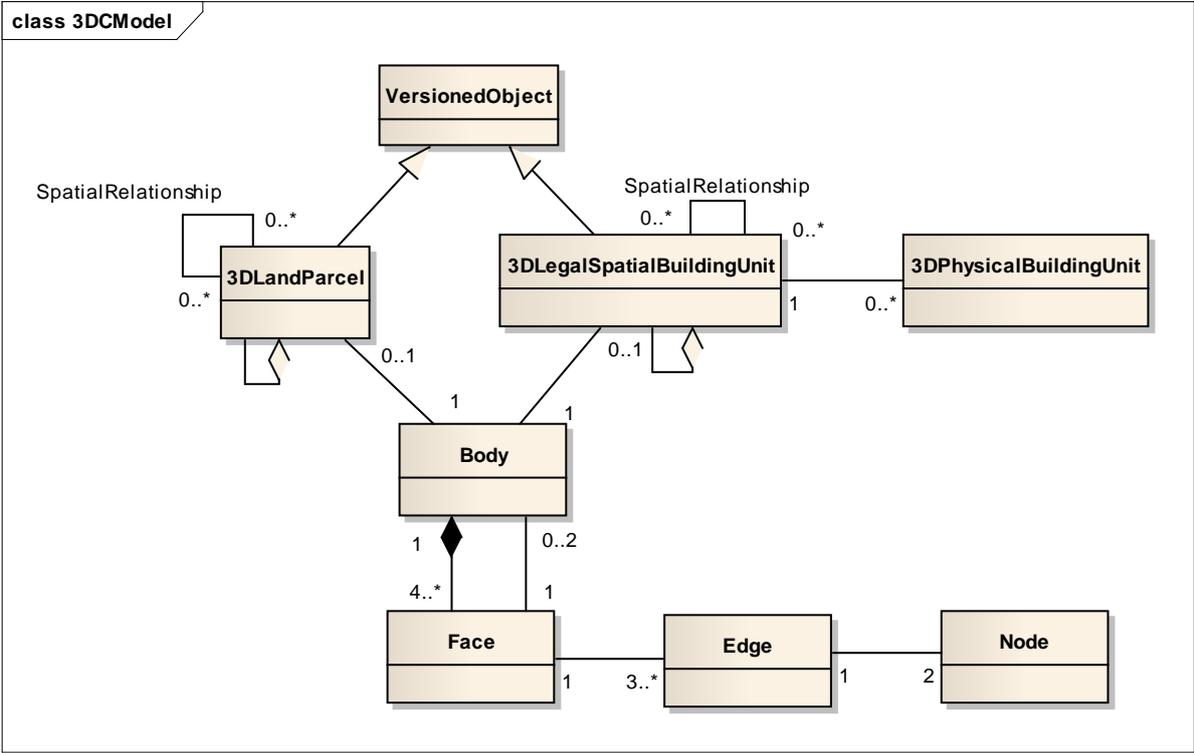
Figure 2. Data model in prototype system
