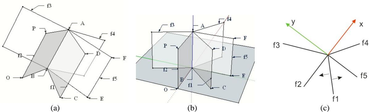
Figure 8. Face-sorting based on shared edge
