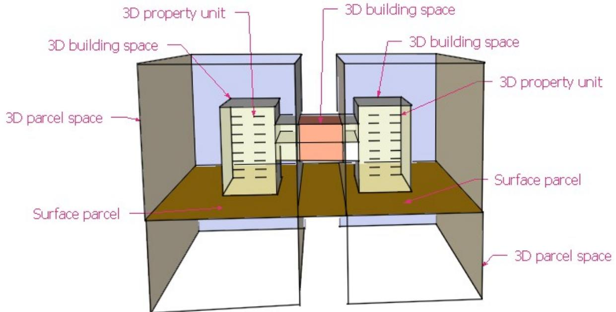
Figure 3. Different 3D spaces in 3D cadastre (modified from (Guo and Ying, 2010))
