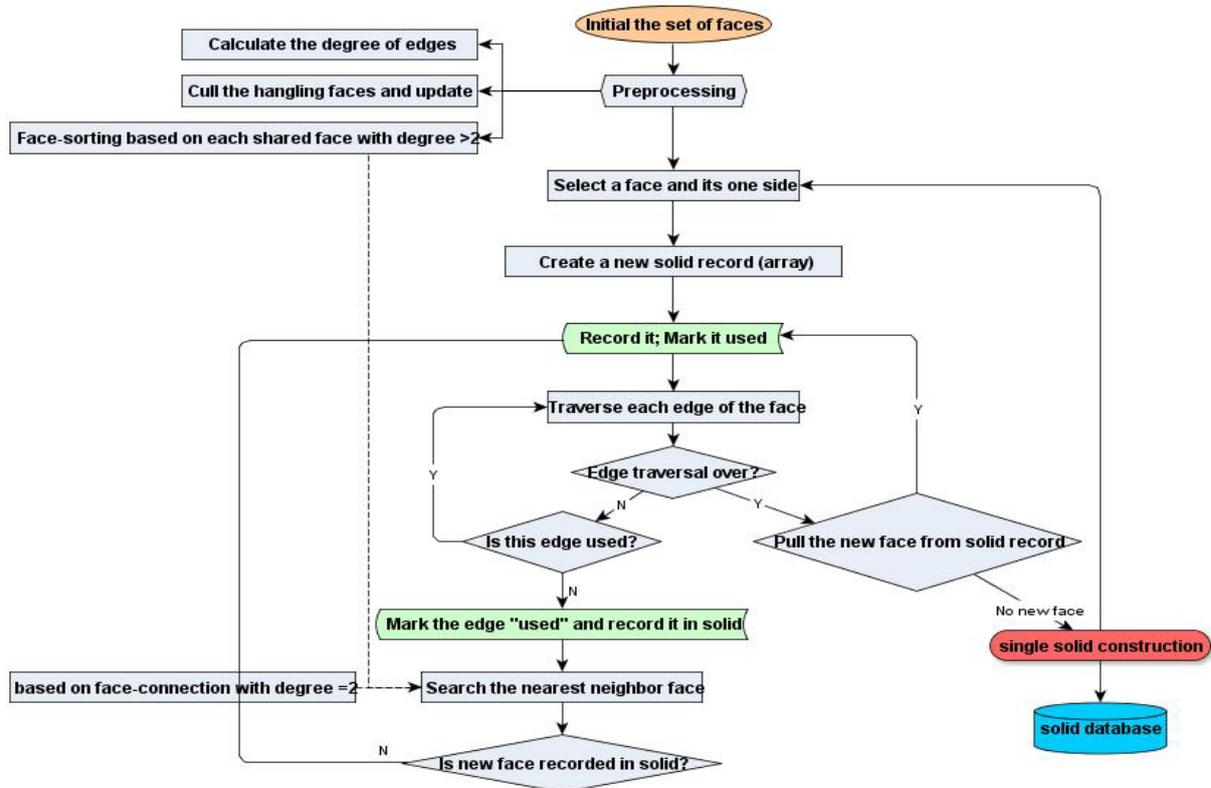
**Figure 10. Workflow of the automatic construction of the valid solid based on shared edge**
