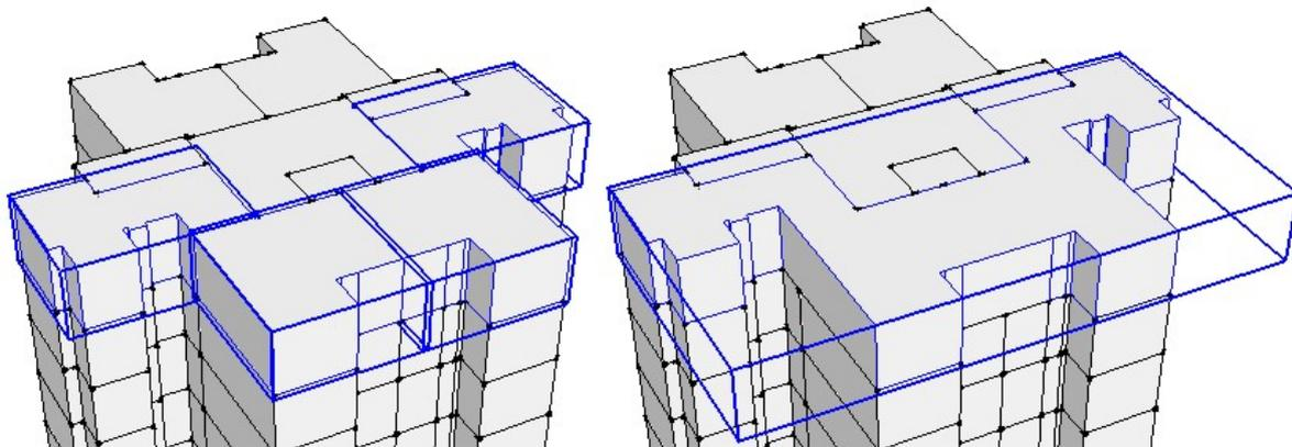
**Figure 16. Mergence operator of four bodies**
