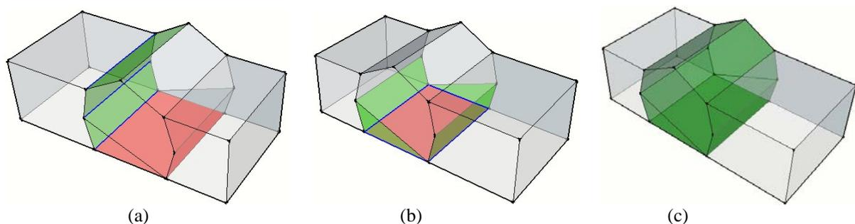
**Figure 9. Different shape during the process: a) the strip zone based on DSF; b) the surrounding shape based on BSF; c) resulting solid**
