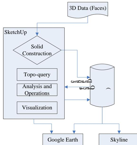
**Figure 14. Framework of the prototype**
