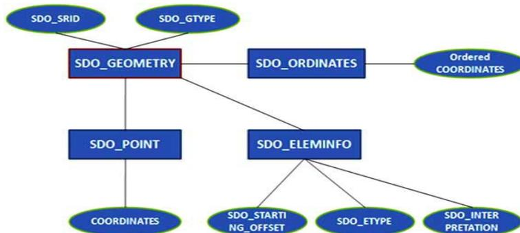
Figure 5. Decomposition of the SDO\_GEOMETRY data type
