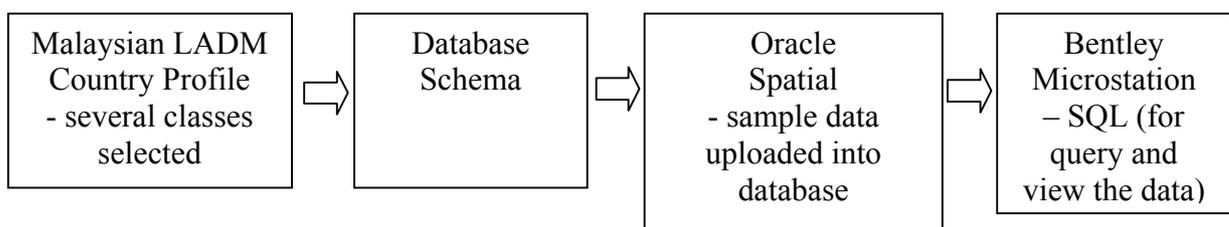
**Figure 5: The four steps of the prototype development**
