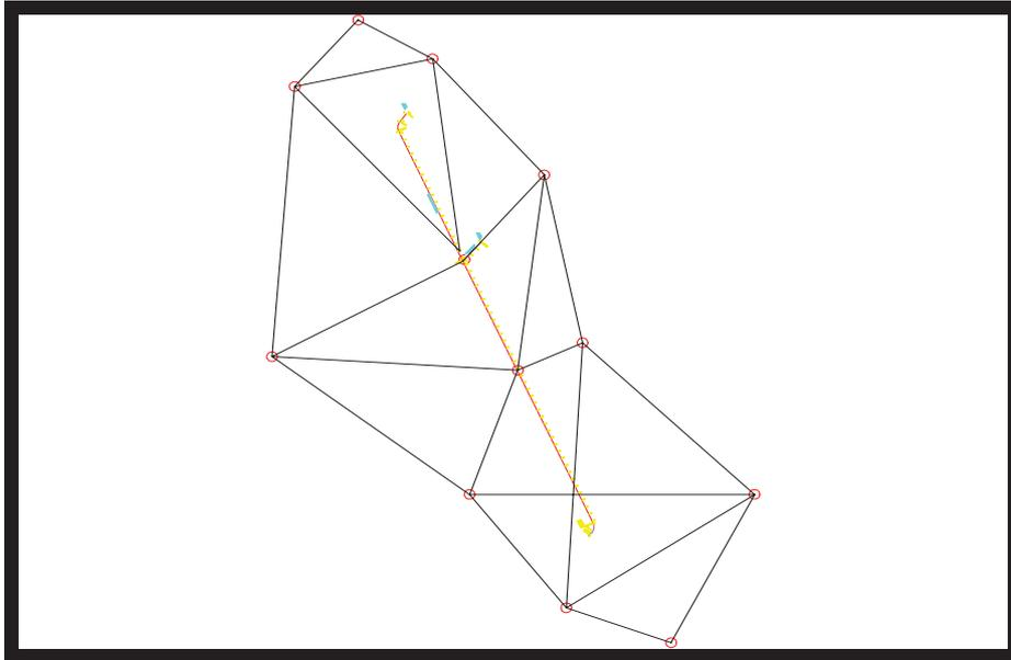
Figure 3 Horizontal network of hydropower system "Dabar"
