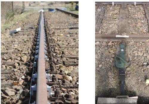
Fig. 13 Fiber optic setup and lateral deformation using a winch for simulating natural events
