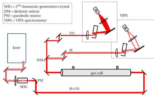
**Fig. 2** The setup uses an IR FC laser source. Visible light is created by focussing on the second order nonlinear crystal. IR and VIS share the same beam path until they are separated by a dichroic mirror guiding each of them to the respective spectrometer
