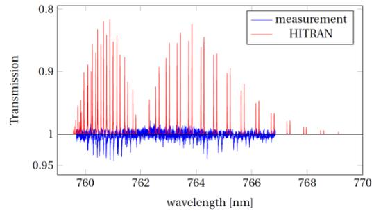
**Fig. 6** Measured line spectrum for 1.5 m light propagation in  $O_2$  at  $27^\circ C$  and atmospheric pressure. The measured transmission is off by a factor of 4 with respect to the expected results as well as showing a noise level that forbids temperature estimations.
