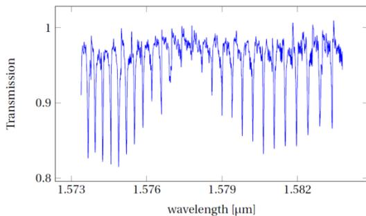
**Fig. 5** Measured line spectrum for 1.5 m light propagation in  $CO_2$  at  $27^\circ C$  and atmospheric pressure. The signal shows fluctuations up to 5% at the baseline preventing temperature estimations.
