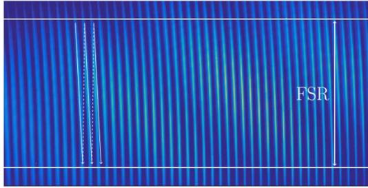
**Fig. 4** Typical camera image of broadband laser passing through a VIPA spectrometer. Information is contained within the FSR length of one VIPA line. To access a broader range the neighbouring lines have to be concatenated.
