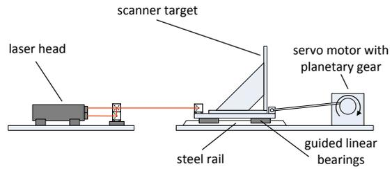
Fig. 1 Diagram of the oscillation table
