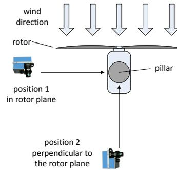
Fig. 5 Measurement configuration, top view
