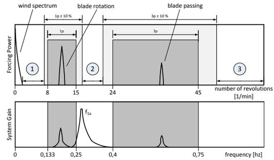
**Fig. 2** Forcing power and system gain
