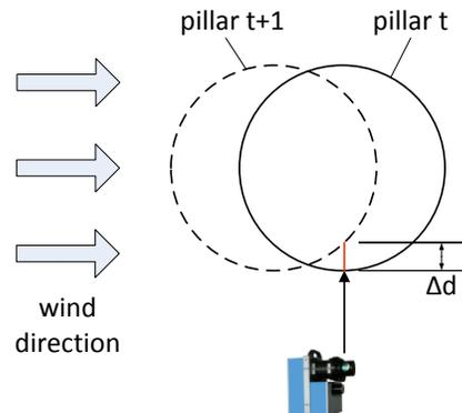
**Fig. 9** Cross section pillar, time t and time t+1
