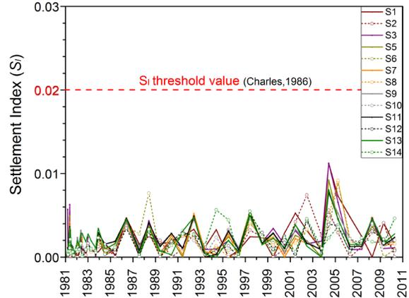
**Fig. 4** The settlement index of the crest control points of Pournari I dam has never exceeded the threshold value of 0.02 from 1981 until 2010.
