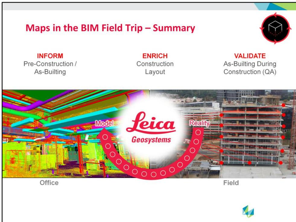
Then new construction layout information from the office is replicated on the job site using total stations – bringing the model into reality or physical construction [animation3] And then new construction in the field is captured using scanners and total stations so the office can validate what was built is what was designed – bringing reality in the field back to the model in the office.
