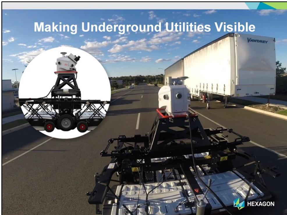
Perhaps you need to move from hard to see objects to impossible to see objects, simply because they are underground. With a combination of LiDAR and radar technology we developed a system which can see the unseeable...
