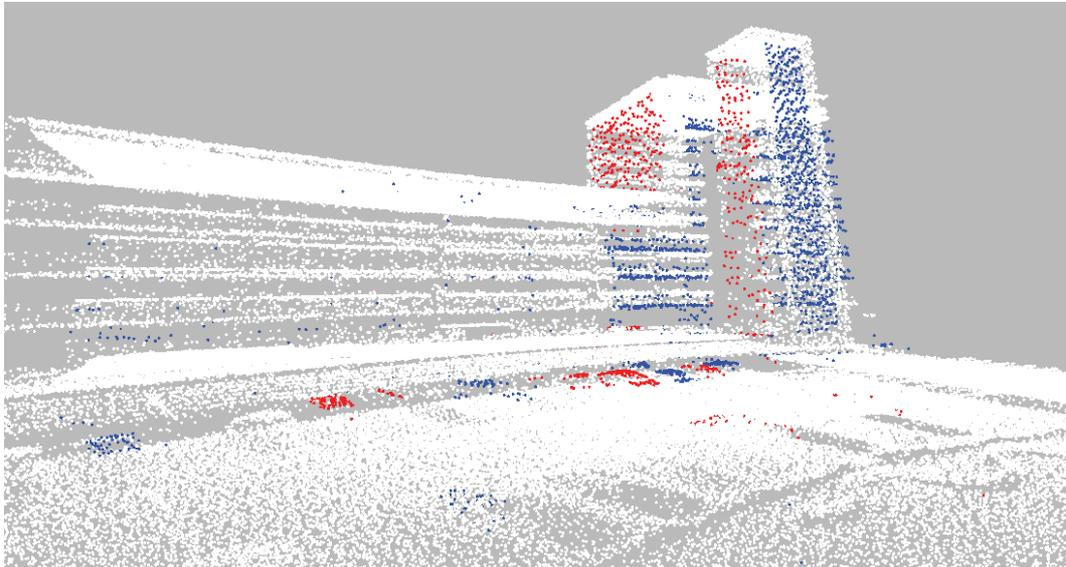
**Figure 6. Detected changes due to differences in the viewing angle**
