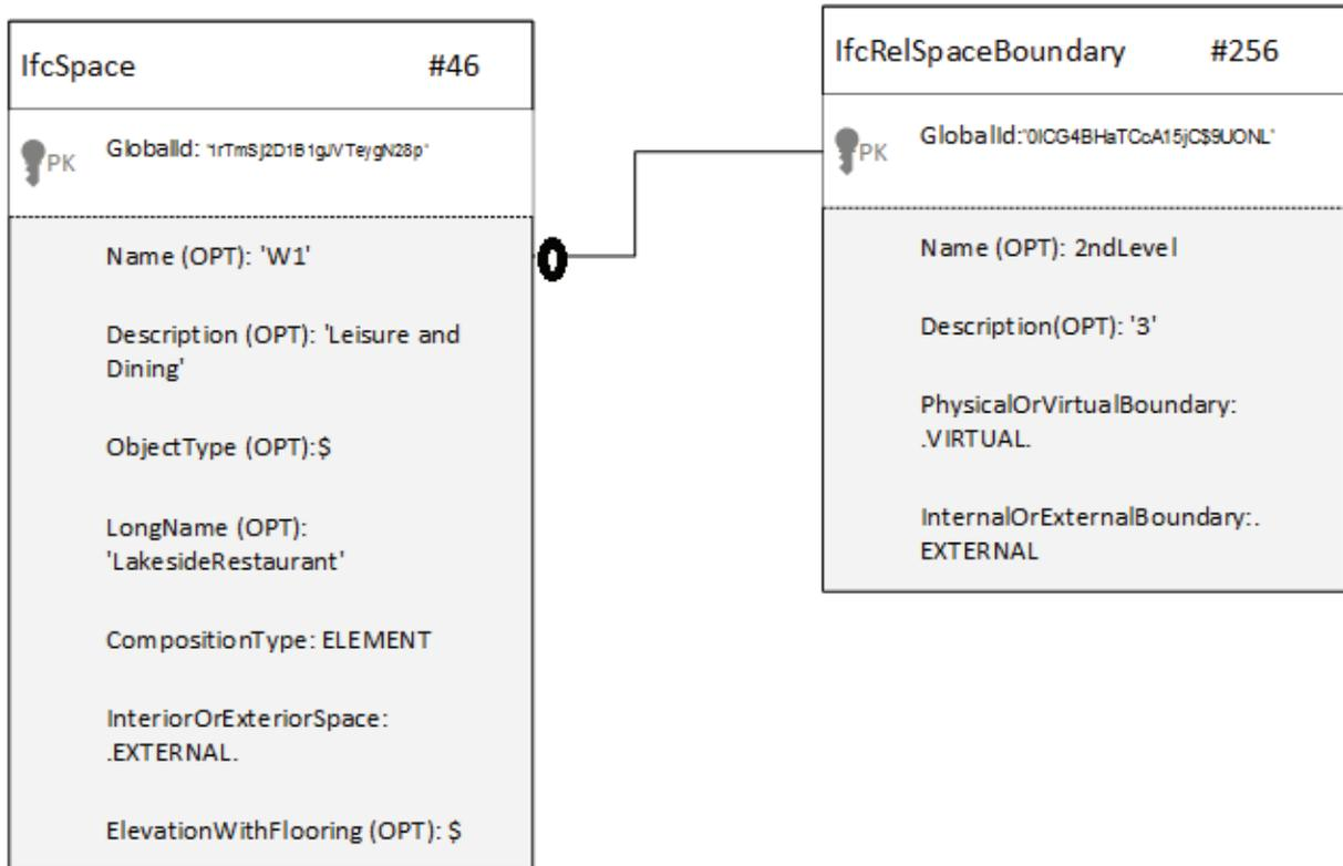
Figure 9. Extract from IFC model showing *IfcSpace* with attributes for a conceptual mass of the Lake Restaurant. The '3' in the *IfcRelSpaceBoundary* entity represents a proposed new description for an ambulatory boundary and replaces the original '2a'
