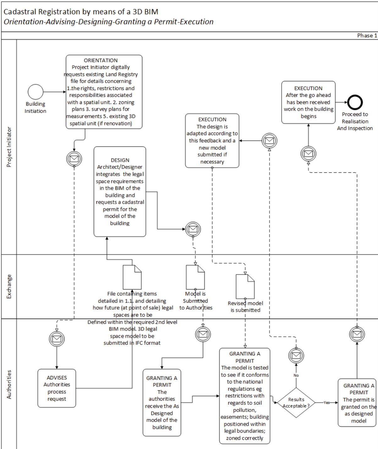
Figure 10 IDM Workflow: Cadastral Registration by means of a 3D BIM Phase 1
