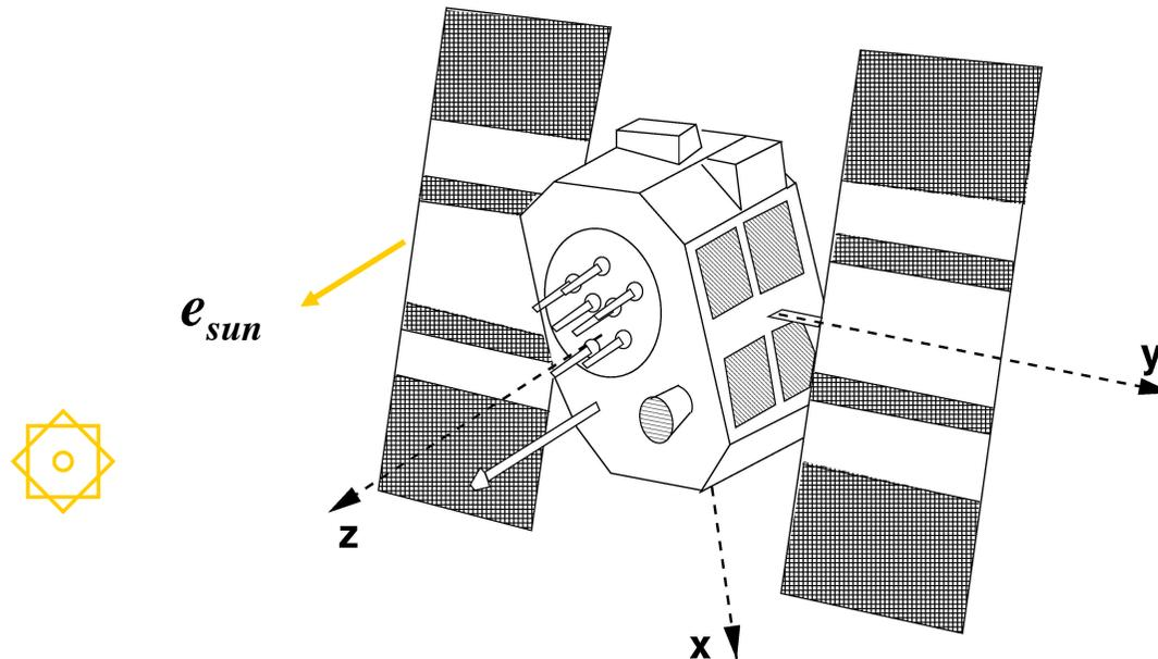
Satellite-fixed Cartesian coordinate system  $(x,y,z)$ , unit vector  $e_{sun}$  pointing from satellite to Sun is perpendicular to solar panels under Yaw-steering, where z-axis points to Earth, y-axis is perpendicular to  $e_{sun}$ .
