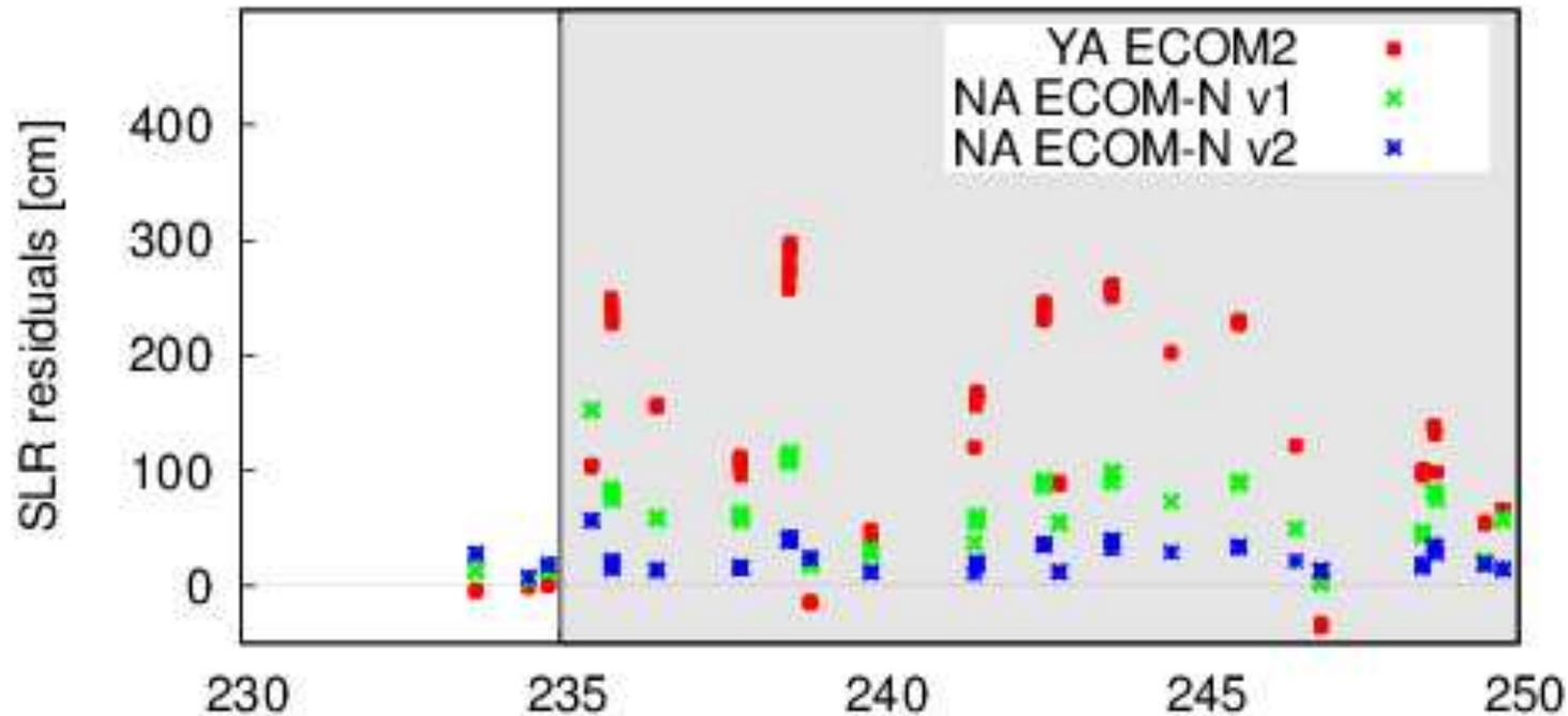
Yaw-Steering SRP (red) is not sufficient for ON mode
