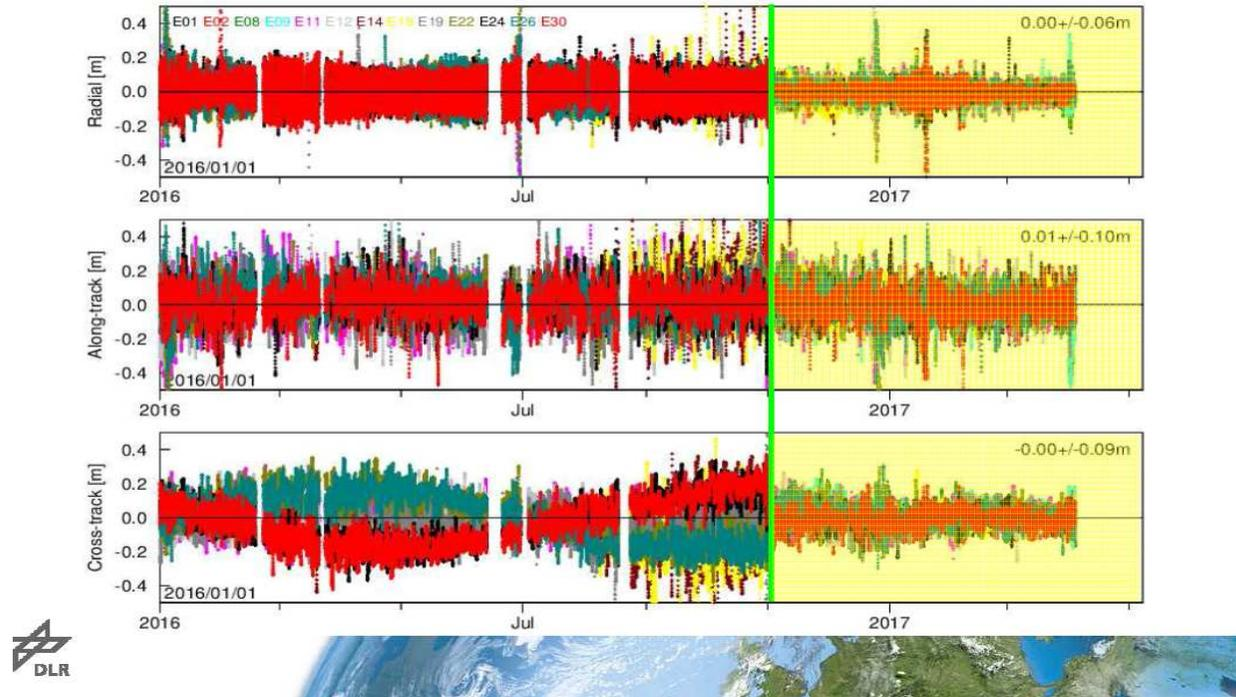
Documentation of an orbit model change by Wuhan AC towards end of 2016. Much improved consistency in 2017 (from Steigenberger & Montenbruck (2017)). **Example illustrates consequences of incorrect/missing GNSS-metadata.**
