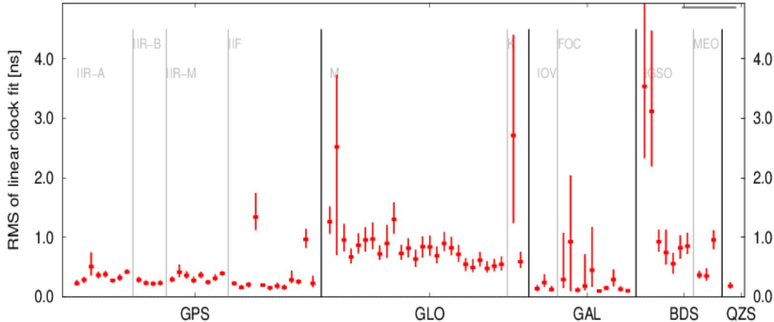
**Satellite orbits may also be validated by satellite clock corrections for those satellites which have high-accuracy oscillators. Figure shows the median of the daily RMS of clock estimates w.r.t. linear clock models for different satellite types. Large values indicate modeling problems and/or actual clock quality problems (Prange et al. (2017))**
