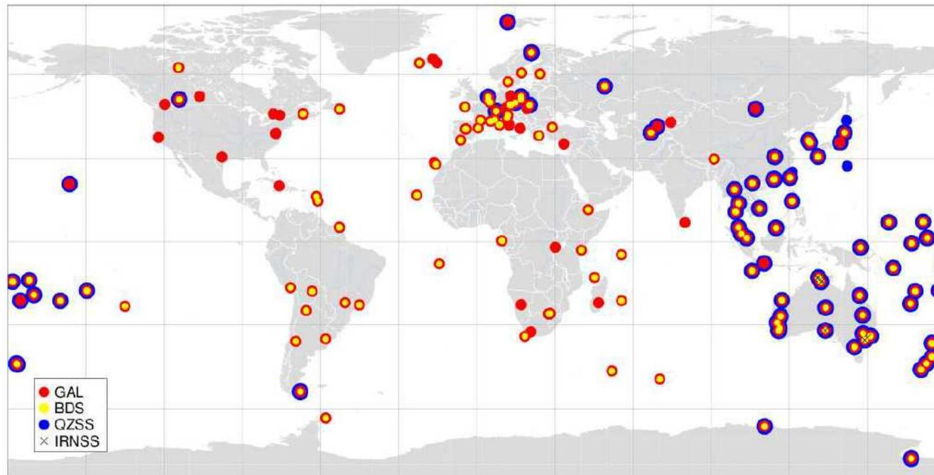
**Currently, about 190 Multi-GNSS stations track a combination of Galileo, Beidou, QZSS, in addition to GPS and GLONASS (from Steigenberger & Montenbruck (2017) ).**
