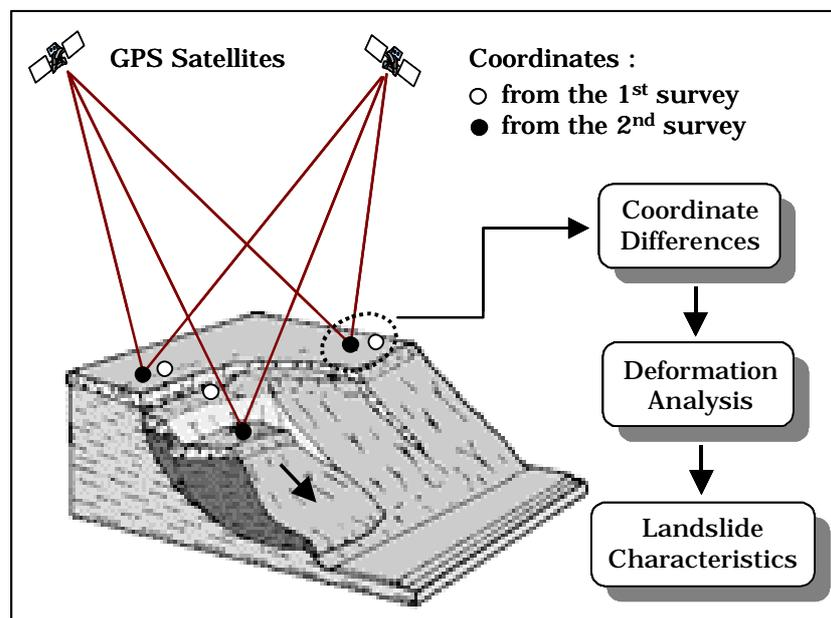
**Figure 2:** Principle of GPF Survey Method for Landslide Monitoring.
