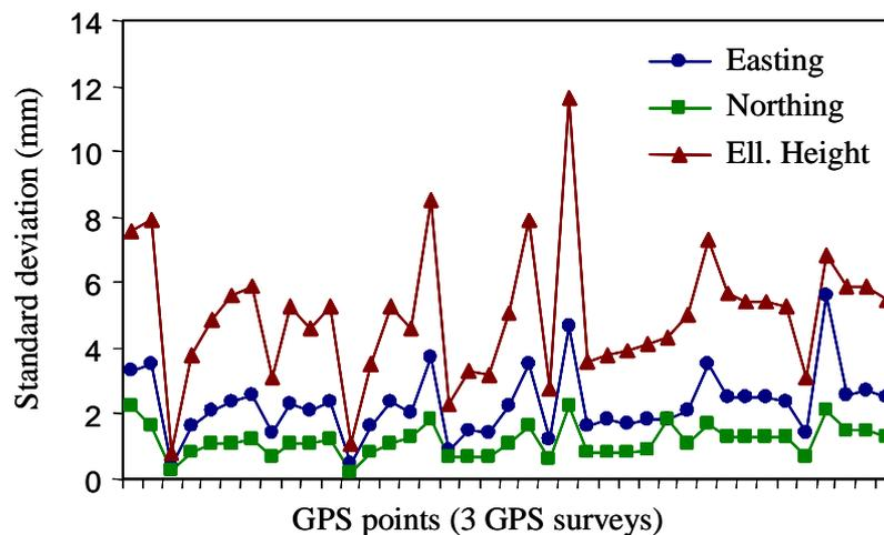
**Figure 5:** Typical standard deviations of the estimated GPS coordinates obtained from three GPS surveys. GPS
