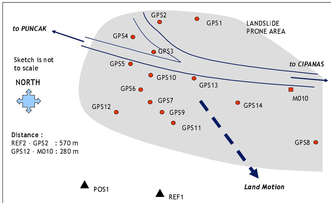
**Figure 3:** Landslide GPS monitoring network in Ciloto (West Java, Indonesia).
