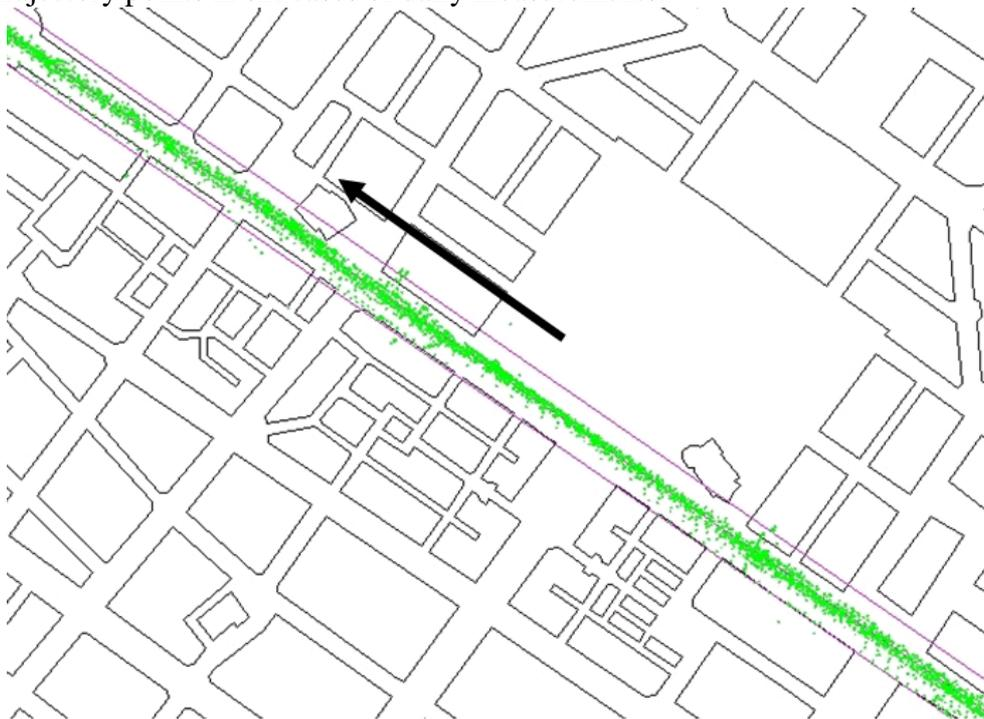
**Figure 1.** Stand-Alone GPS points distribution along the road segment under consideration in the EW direction
