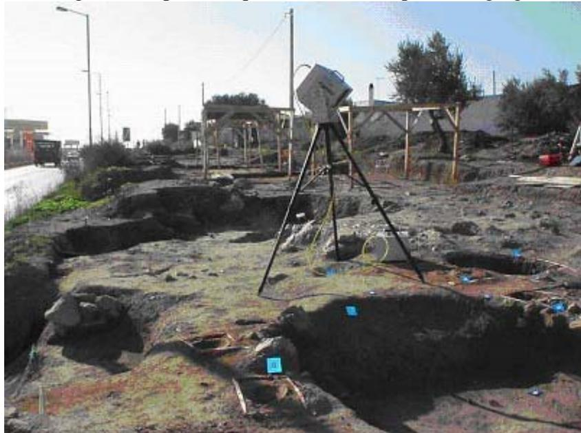
**Figure 3.** Laser scanner facing the cavities
