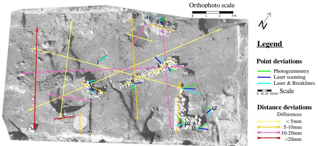
**Figure 10.** Accuracy check using point and distance deviations (based on orthophoto-mosaic A)
