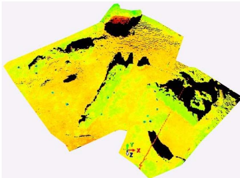
**Figure 5.** Snapshot of registered point cloud of the excavation site
