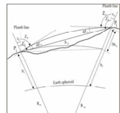
Figure 4. Survey model of the reciprocal trigonometric levelling
