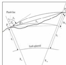
Figure 3. Survey model of the unidirectional trigonometric levelling
