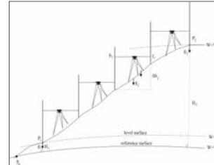
Figure 2. The survey model of the geometric levelling
