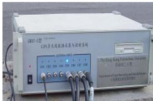
**Fig 2.** GPS multi-antenna control unit
