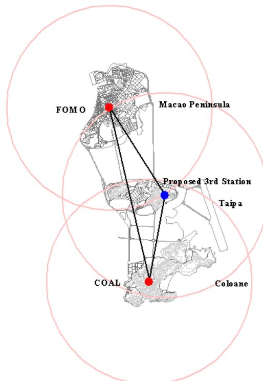
**Figure 7.** Redundancy coverage area with three reference stations
