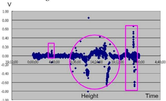
C. Coordinates differences between static GPS and single RTK in Height direction
