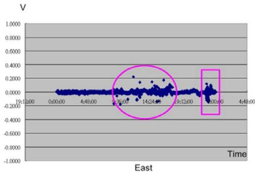
A. Coordinates differences between static GPS and single RTK in East direction
