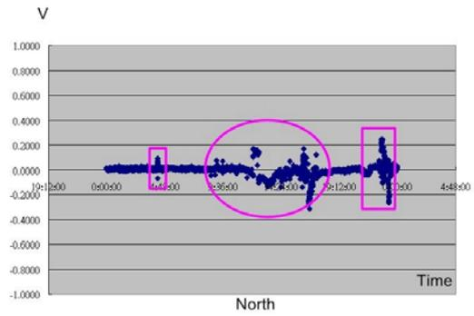
B. Coordinates differences between static GPS and single RTK in North direction
