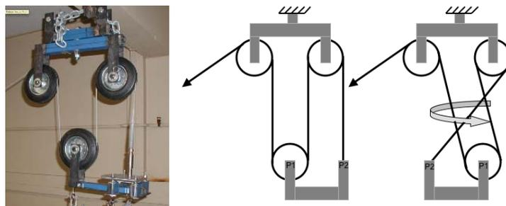
**Figure 9:** Pulley system and cable twisting
