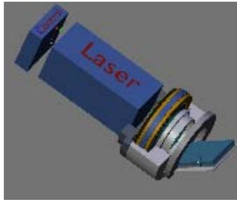
**Figure 11:** Model of laser and rotating mirror assembly
