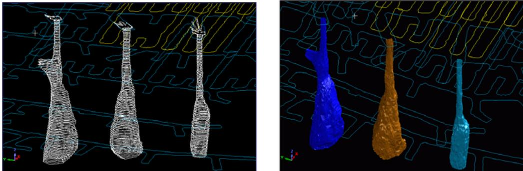
**Figure 16:** Ore Pass a) Wire Frame and b) Rendered Solids
