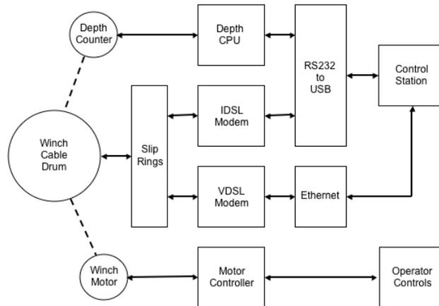
**Figure 3:** Winch block diagram
