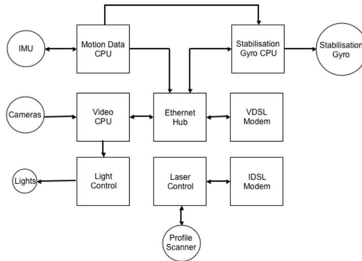
**Figure 5:** Pod component sub processors
