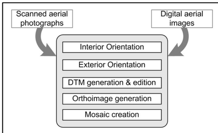
Figure 1. Orthoimage generation process
