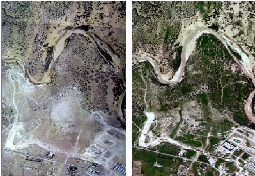
**Figure 3. The two generated orthoimages mosaics from scanned photographs (at left) and from numeric images (at right)**
