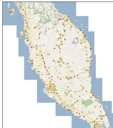
GNSS observations with RTK technique involving a total number of 77 bench marks (BM)
