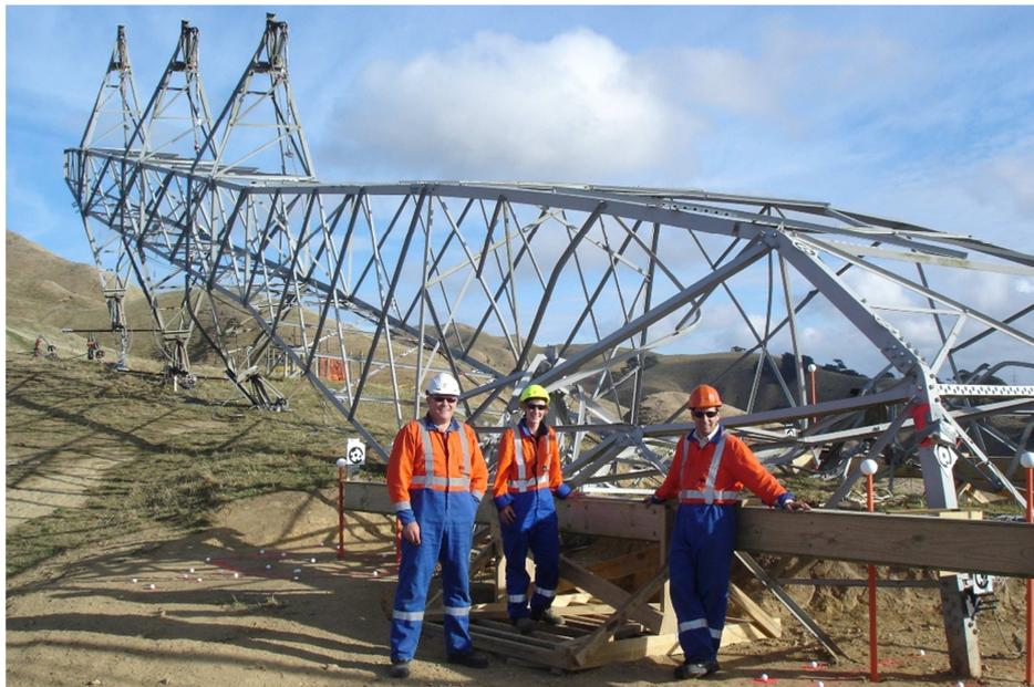
*Figure 1 – The decommissioned tower T26 after the pull-over test*
