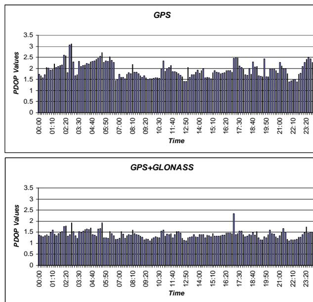
Figure 1. GPS and GPS/GLONASS PDOP values
