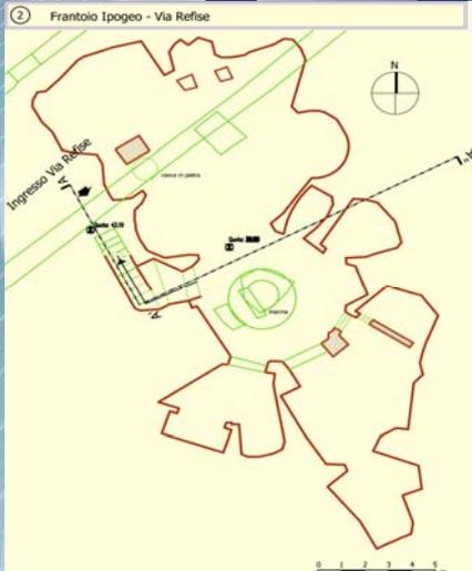
The secondary corridors leading from the main cavity, were measured trilaterally and radially with a laser meter. The reference points used for the radial measurements had been previously defined with the total station laser
