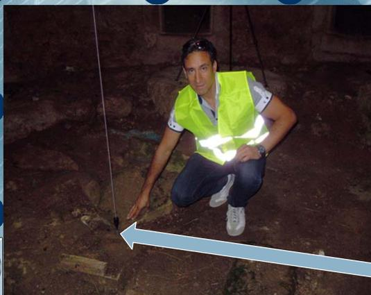
*The main feature of the traverse has been to have some points hooked to the points which were detected with the GPS described above, and carefully screened on the floor inside the hypogeum with a proper plumb-line.*
