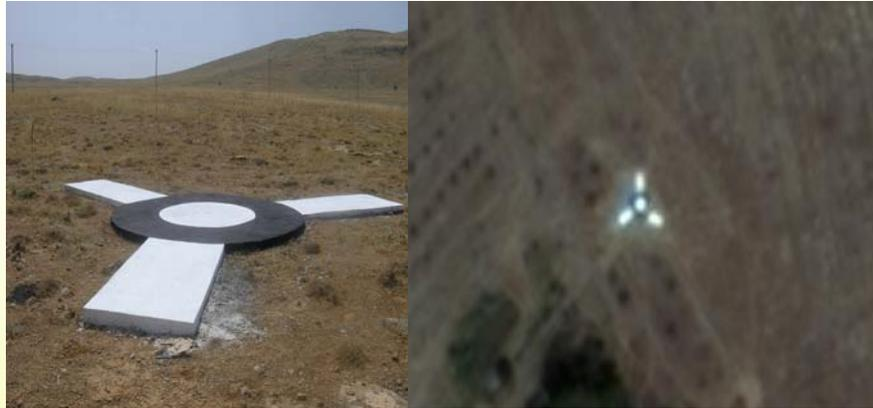
a) The GCP on the field      b) The GCP on the image
