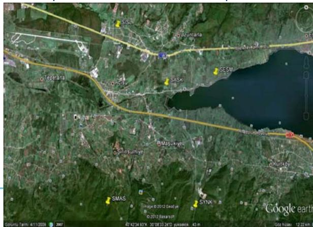
Employing GPS observation techniques has led us to concentrate on two network points, one on each side of the fault, chosen for their best descriptive characteristics of the fault, namely SISL and SMAS. Besides, SESM and SYNK points have attained narrow signal clearance sight to GPS satellites over the years because of overgrowing vegetation and trees
