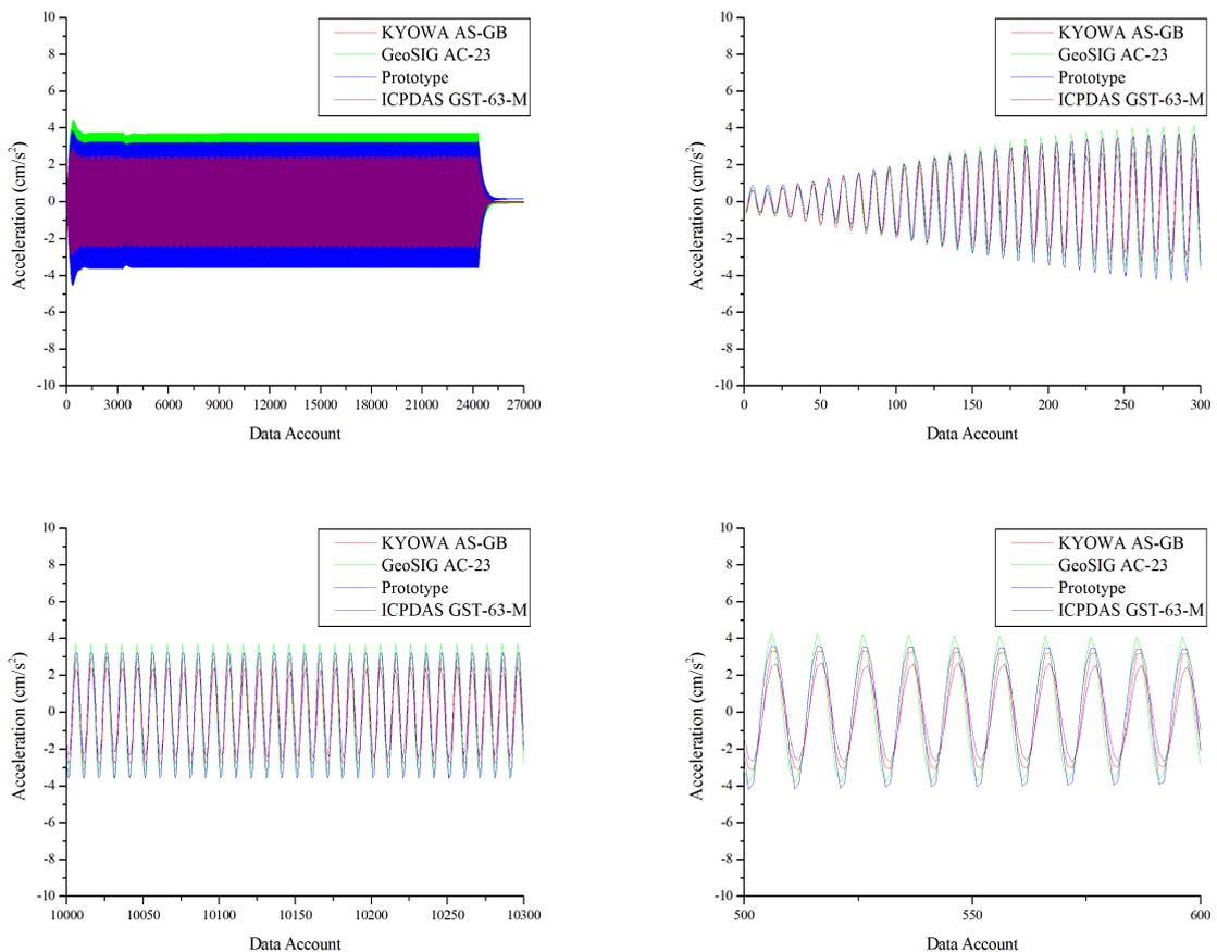
Figure 12. Time series data of accelerometers (10Hz, 4gal)
