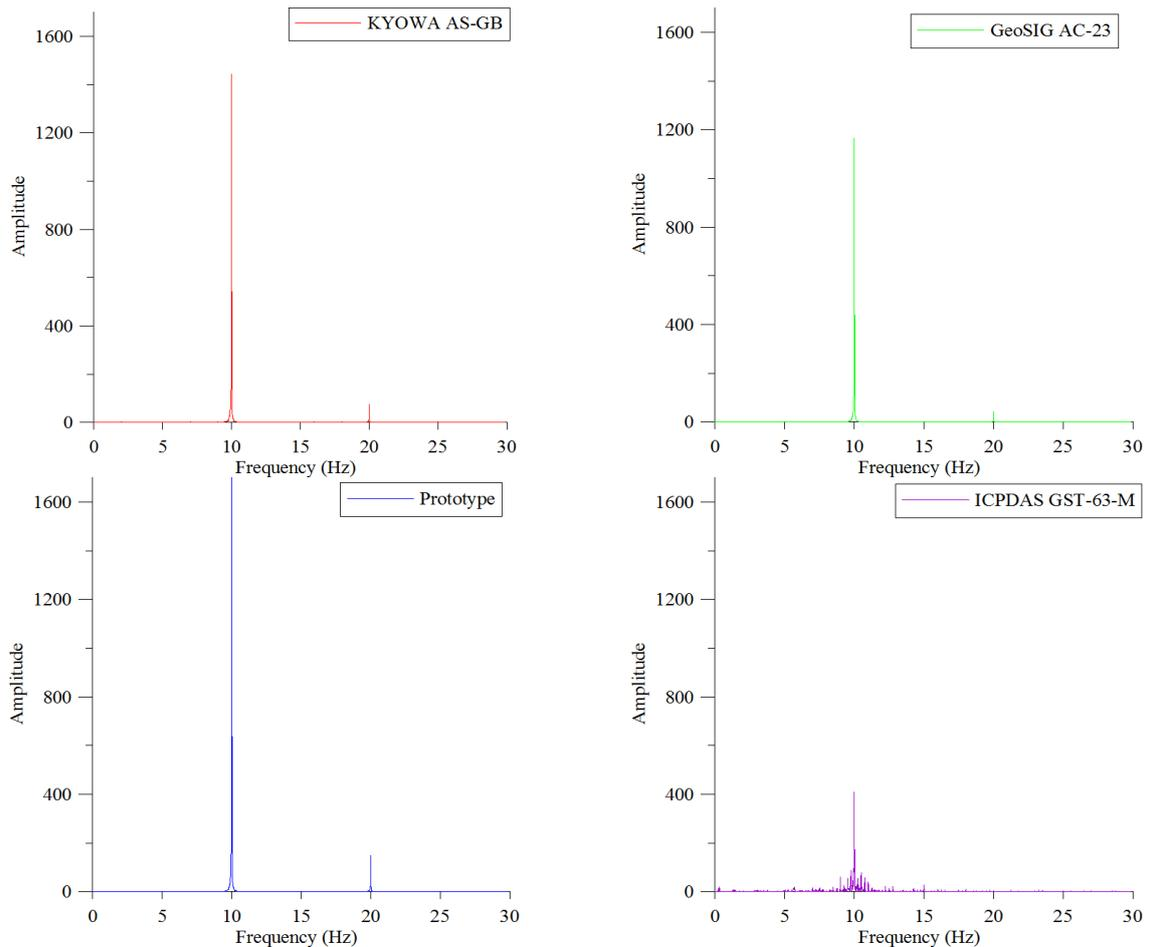
Figure 13. Results of FFT analysis (10Hz)
