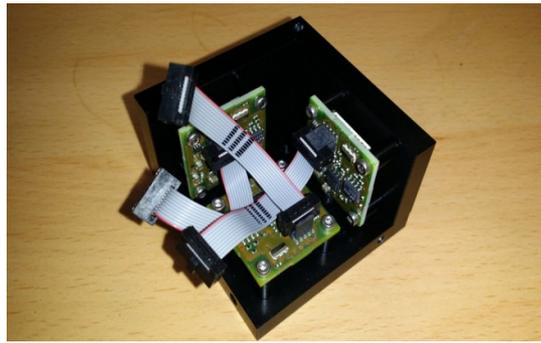
Figure 5. Inner structure of the sensor module
