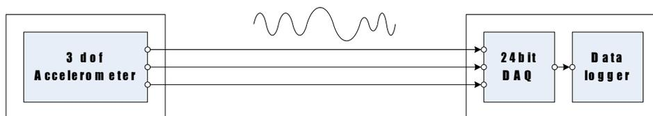
Figure 3. Existing analog output type
