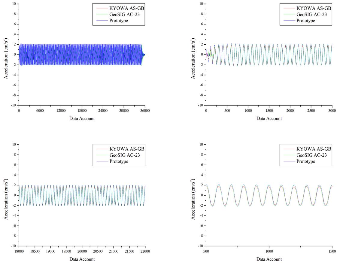
Figure 10. Time series data of accelerometers (1Hz, 2gal)
