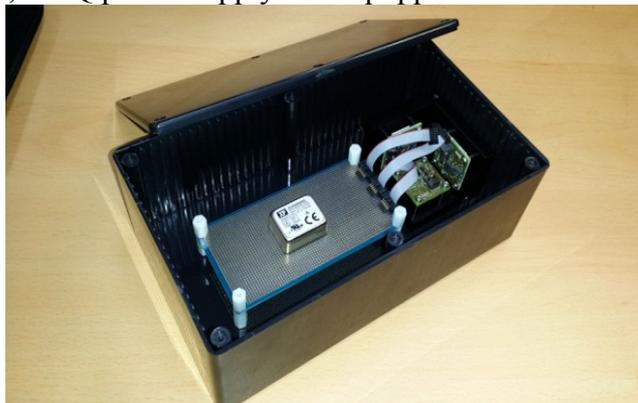
Figure 7. 3-axis accelerometer of digital output type
