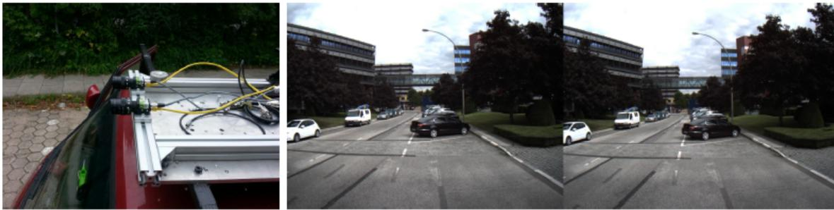
**Figure 5** Stereo camera system, the view from both cameras
