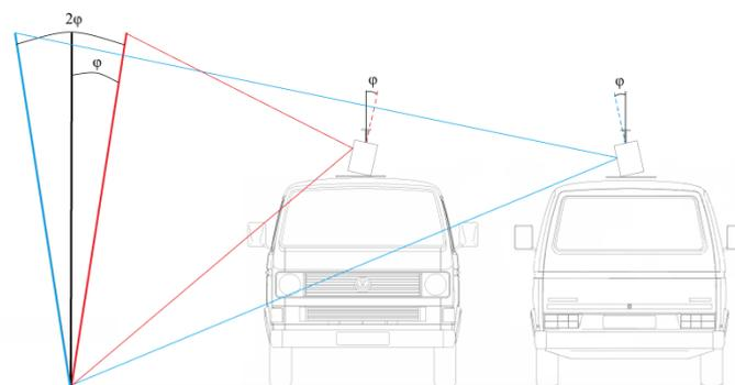
**Figure 7** Effects of a faulty Roll-angle. Recording of an object with two rides on the same trajectory with same speed (according to Keller and Sternberg, (2013)).
