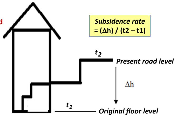
Figure 3. Principle of geometric-historic method for land subsidence estimation, for the cases of bridge and house affected by land subsidence (upper and lower sketches).
