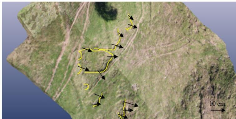
**Fig. 12:** Sliding locations and velocity vectors in 3D model of sub-area #4
