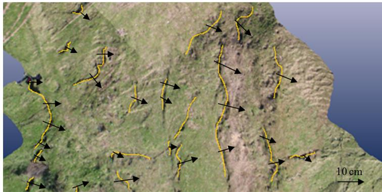
**Fig. 11:** Sliding locations and velocity vectors in 3D model of sub-area #1
