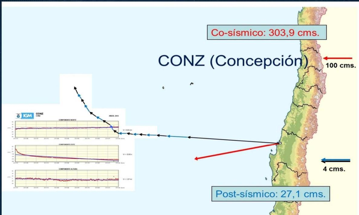
Post-seismic movement of CONZ station in Chile up to the year 2013
