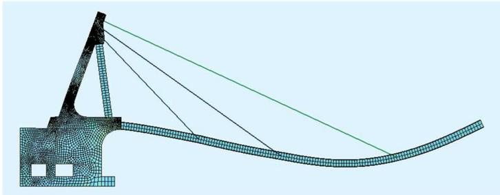
vertical displacements of deck under maximum static loads
