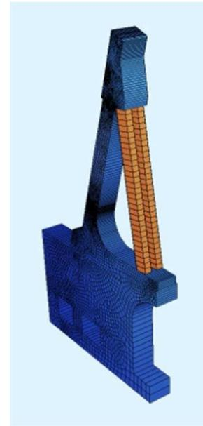
finite element mesh of pylon
