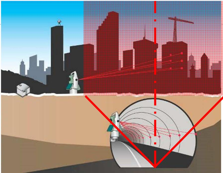
When excavation is conducted to lead underground connections such tunnels and galleries the ground level is subject to subsidence impacting the infrastructures like buildings, bridges, pipe lines and roads...
