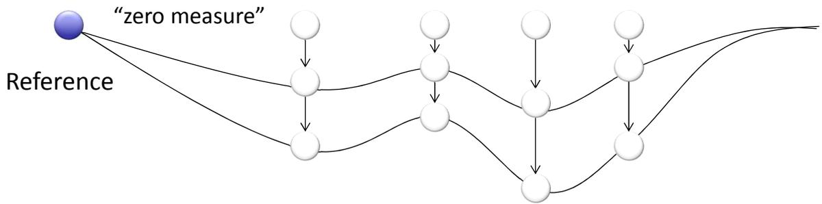
The measure is obtained by reading the pressure of a special fluid contained in a pipe. In particular, the displacement between two sensors is proportional to the pressure difference.
