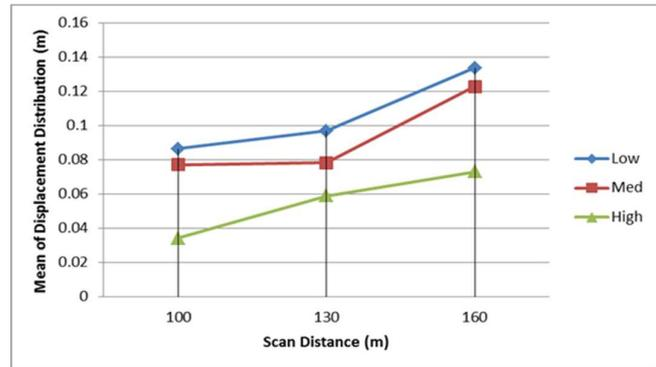
Plot for mean of displacement distribution versus scan distance for three different scan resolutions
