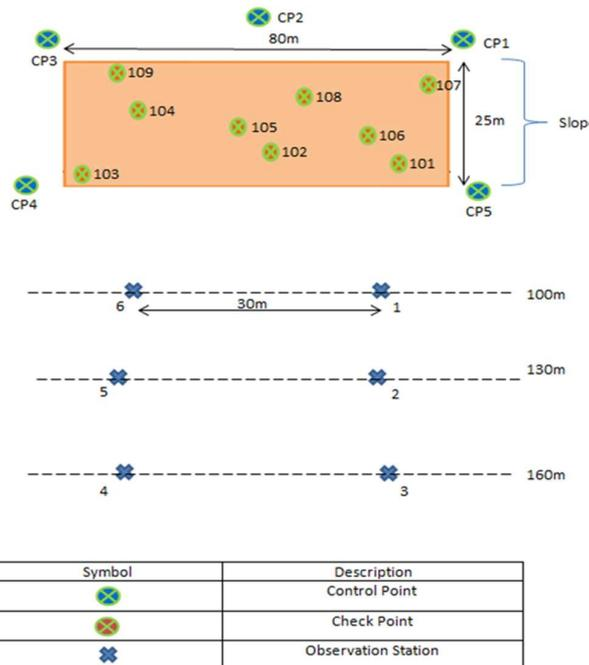
Overall layout of the control points, check points and observation stations
