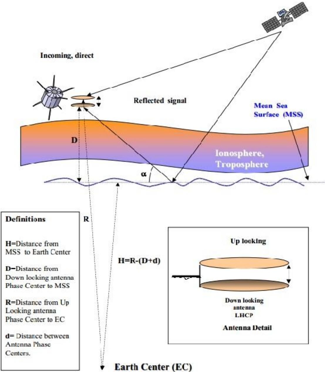
Fig 2: Measurement of scattered signal (Ruffini et al., 2000)
