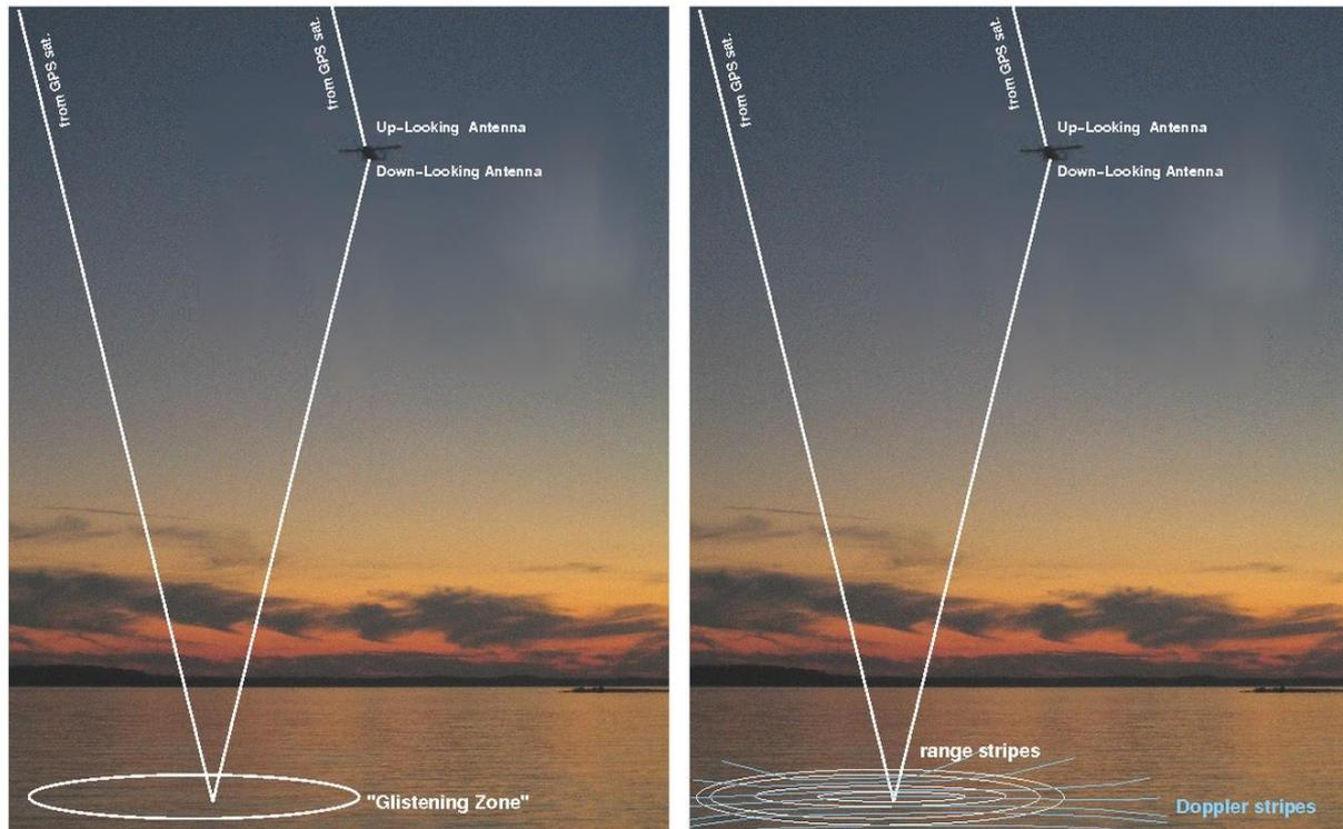
Fig 1: GNSS-R measurement concept (IEEC,2015)
