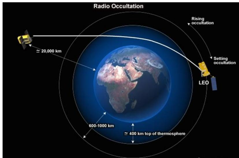
Fig 7: GNSS-RO principles and geometry (EUMETSAT)
