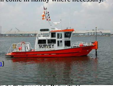
Figure 4: Hydrographic Charting Vessel (<http://www.hydrosurveys.net/surveys.htm>)
