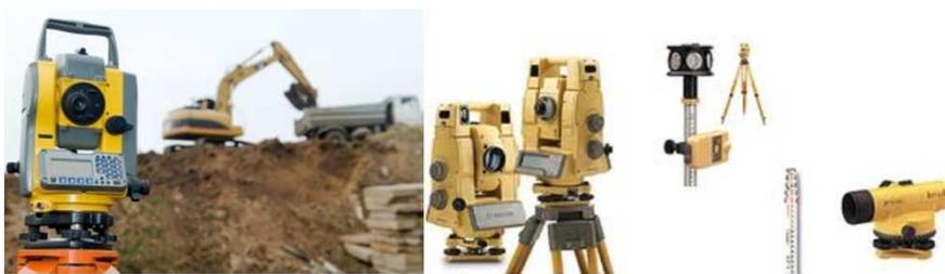
**Figure 3a:** Electronic Total Station, Theodolite and Laser Levels for Precise Engineering Surveys
