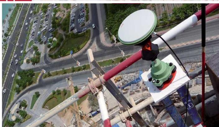
Fig. 12a: Monitoring Vertical Towers with Core Wall Control Survey System (CWCS) (Source: van Cranenbroeck (n.d))
