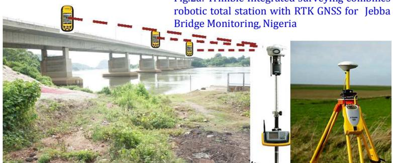
**Fig.2a:** Trimble Integrated surveying combines robotic total station with RTK GNSS for Jebba Bridge Monitoring, Nigeria
